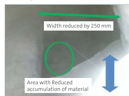
Top view of cyclone: Red mark plate shows new modification implemented
